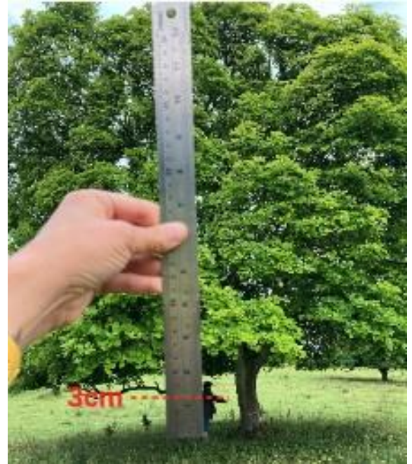
Figure 3: Guide the second person to point out on the tree trunk the point that lines up with 3cm on the ruler.
